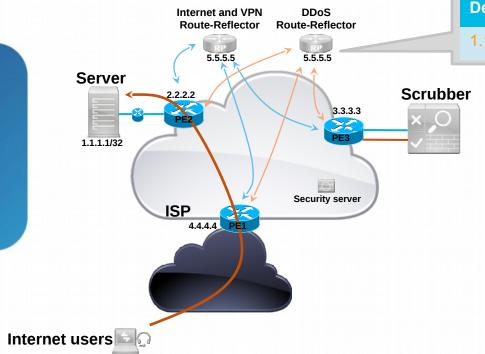
**Destination Next-hop** 1.1.1/32 3.3.3.3 DDoS Route-Reflector was pre-٠ visioned Mitigation route to 1.1.1.1/32 is ٠ injected on the DDoS RR by the Security server
